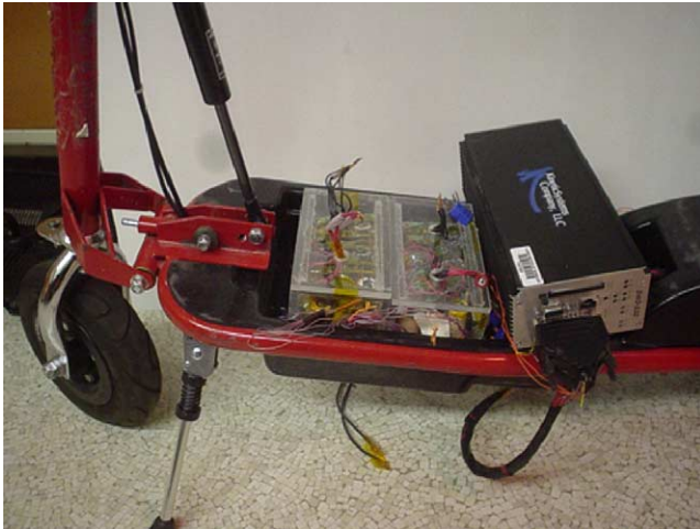
Fig. 3. Assembly of two Li-ion battery modules and data acquisition (DAQ) system in Zappy electric scooter.
